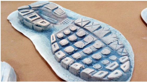
Figure 7: Casts are created of footwear impressions to preserve them and allow for comparison and analysis. (Courtesy: NFSTC)
