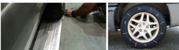
Figure 5: A reference print from a tire is captured by inking the tire and driving overpaper. (Courtesy: John Black, Ron Smith & Associates)
