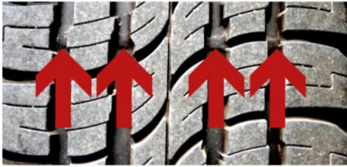
Figure 2: Enlarged image of a tire tread shows characteristics unique to the mold used to create this tire (red arrows). (Courtesy: John Black, Ron Smith & Associates)
